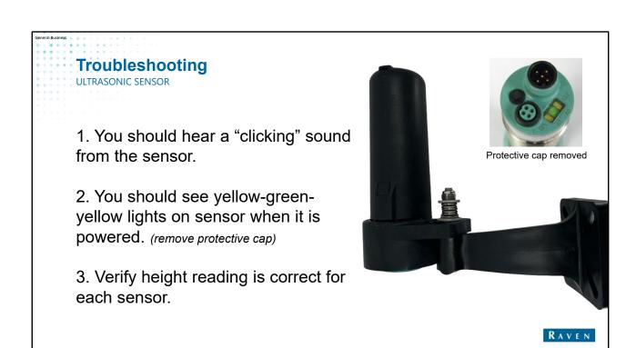
One simple check for the ultrasonic sensors is to make sure you can hear a clicking sound coming from the sensor. This sound means the sensor is receiving power. If it is not clicking, you can remove the protective cap and verify the lights on top of the sensor.
