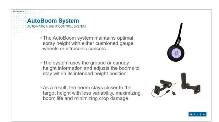
The AutoBoom system maintains optimal spray height with either cushioned gauge wheels or ultrasonic sensors. The system uses the ground or canopy information and adjusts the booms to stay within its intended height position. As a result, the boom stays closer to the target height with less variability, maximizing boom life and minimizing crop damage.
