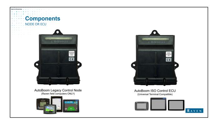
The AutoBoom system comes in two versions, either Raven proprietary CAN bus or universal ISO CAN bus (International Organization for Standardization) which makes it an ideal height control system for most sprayers The terms Node and ECU (Electronic Control Unit) are used interchangeably in some context. Both terms identify a device, microcontroller, that performs specific functions and communicates with other Nodes/ECUs on the CAN bus network.
