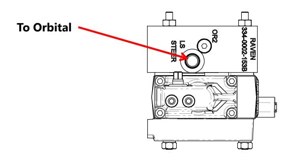
**Logic Cartridge on the Load Sense**
