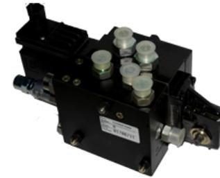
Sauer Danfoss steering valves use voltage control on a single 4-pin Deutsch connector, meaning it will read the machine voltage on the Power pin and supply half of that voltage on the Signal pin for driving straight forward. It will then add approximately 3 volts to steer right at full output, and subtract approximately 3 volts to steer left at full output. It will vary this voltage when steering less than full left or right.
